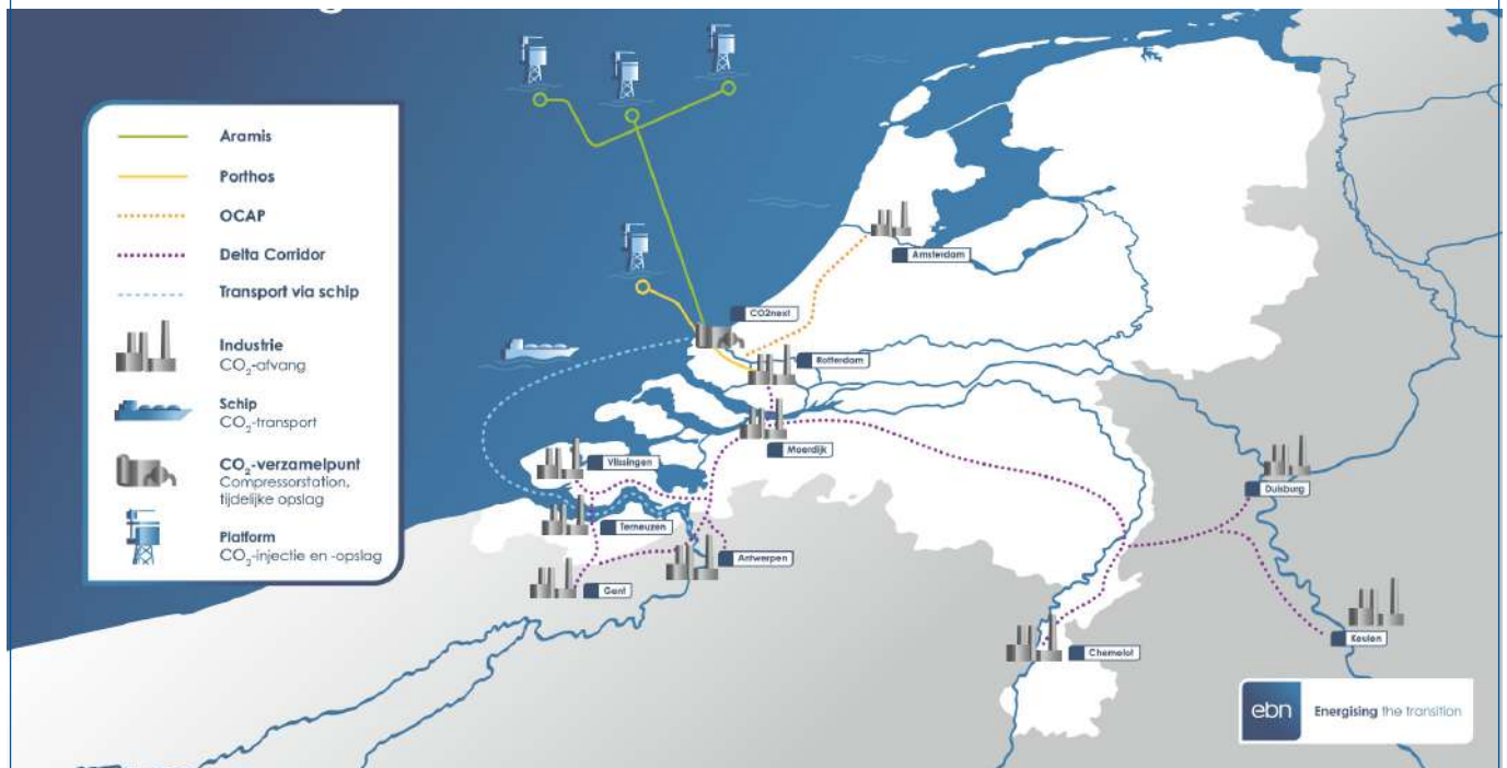
Figure 12: Map of CCS infrastructure in the Netherlands and beyond, including Porthos, Aramis and OCAP
